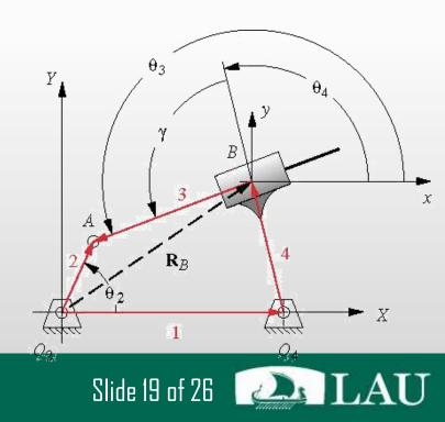
Vector loop equation:  $R_2 - R_3 - R_4 - R_1 = 0$
